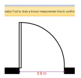
Either accept the suggested measurement or enter another one in the Calibration box. Check your units are correct (m, ft etc) and click OK.
